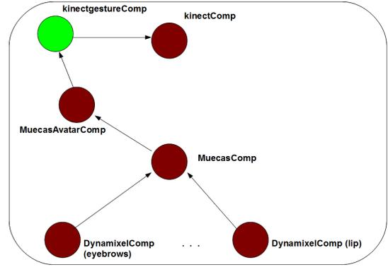
Fig. 7. Dependence Relationships between the different components used in the proposed approach.
