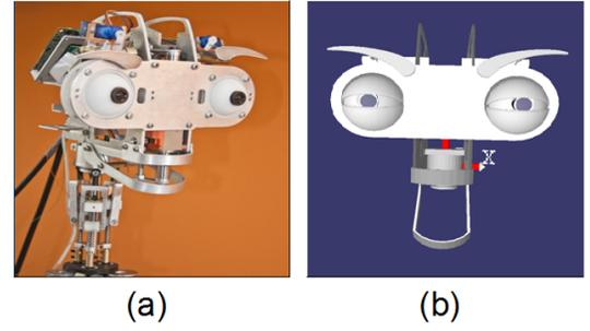
Fig. 5. b) 12DOF Robotics head Muecas; and a) Robotics Head Mueca's avatar.
